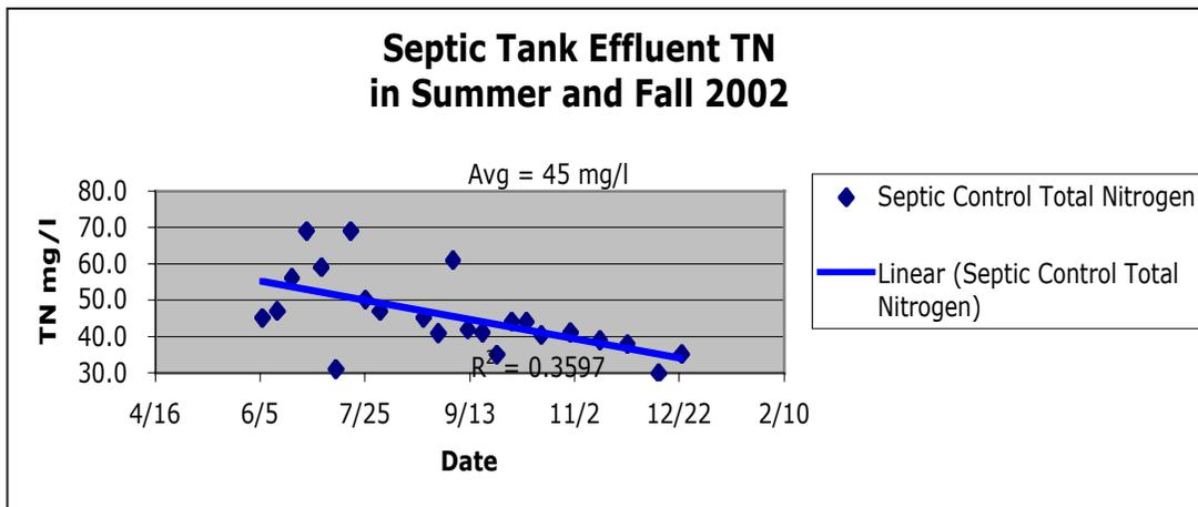
Figure 4c Total nitrogen in septic tank effluent after 24 inches of sand
