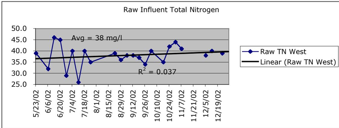
Figure 4b Total nitrogen in septic tank effluent
